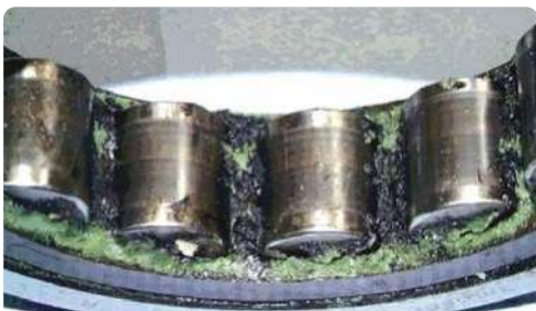
Lubricant degradation caused by electrical discharge currents
