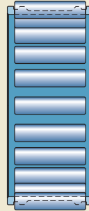
Machined steel cage of the radial bearing
